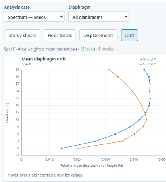
Figure 9. SpecX drift profiles. ETABS maximum drift is left; FEAkalc relative mean diaphragm drift is right. An ETABS axis value of 800 \times 10^{-6} corresponds to 0.08%.
