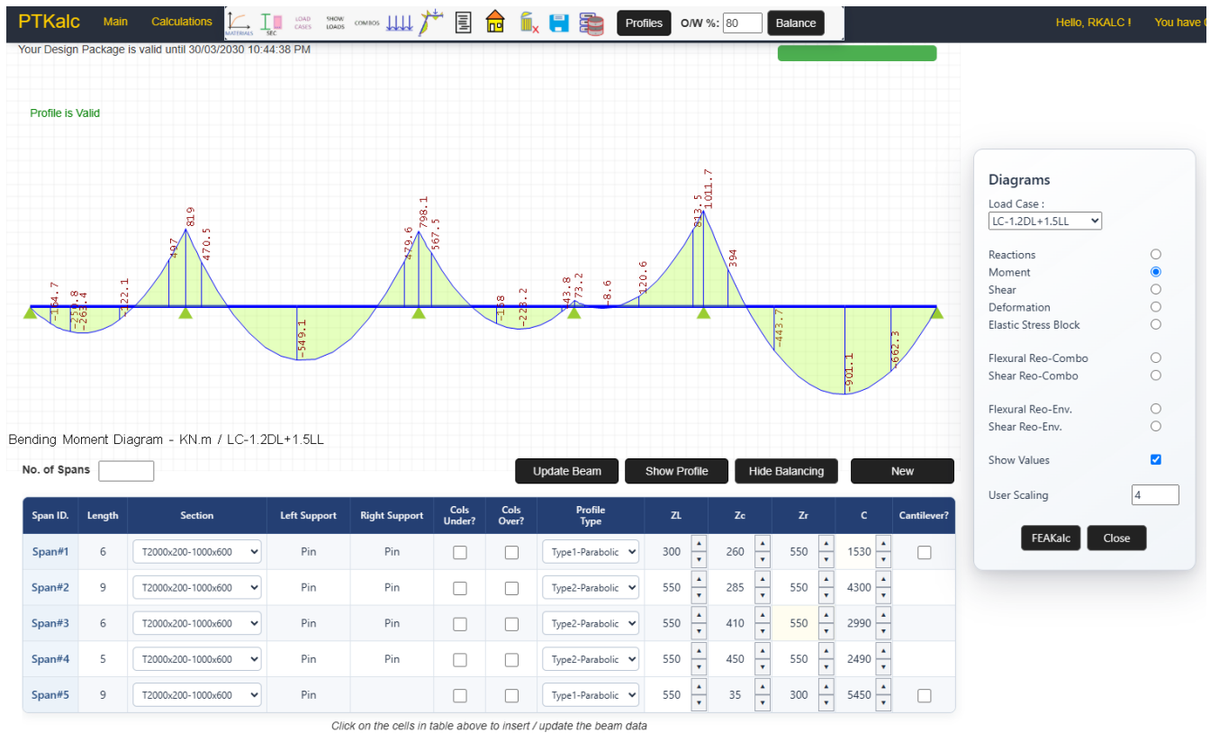
Figure 7 – Showing moment diagrams
